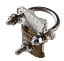
Nominal pipe size range: 3.5" – 4", pipe outside diameter: 3.2" –4.5" Manufactured from electroplated tinned bronze. Conductor range: #6 through 250 MCM PEM stud ensures a flush mounting surface. 5pk.
