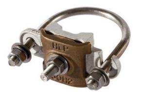
Nominal pipe size range: 3.5" – 4", pipe outside diameter: 3.2" –4.5" Manufactured from electroplated tinned bronze. Conductor range: #6 through 250 MCM PEM stud ensures a flush mounting surface. 5pk.
