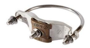
Nominal pipe size range: 3.5" – 4", pipe outside diameter: 3.2" –4.5" Manufactured from electroplated tinned bronze. Conductor range: #6 through 250 MCM PEM stud ensures a flush mounting surface. 5pk.
