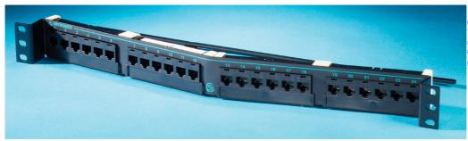
Clarity 5E angled 24-port high density patch panel is cor TIA/EIA Category 5e performance requirements. It occup measures 19" x 1.75". Jacks are grouped in six-port mod Clarity 5E link and channel solution that provides significant performance headroom.
