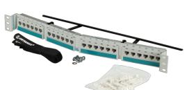
Clarity 6 angled 24-port Category 6 patch panel, high density patch panel is component compliant to TIA/EIA Category 6 performance requirements. White panel occupies 1 rack unit and measures 19"  $\times$  1.75". Jacks are grouped in six-port modules. It is part of the Clarity 6 link and channel solution that provides significant installed performance headroom.
