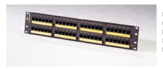
Eight-position jacks, T568B wired to 50-pin female telcos. Legrand® Category 5e 25-pair panels provide a 50-pin connector interface (standard RJ21 wiring) between Category 5e 25-pair cable Gigabit Ethernet hubs requiring full 4-pair cabling. Panels provide front label fields. Use with 845E cable assemblies.
