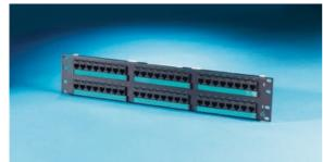
Clarity 5E 48-Port High Density Patch Panel is component compliant to EIA/TIA Category 5e performance requirements. It occupies two rack units, and measures 19" x 3.5". Jacks are grouped in eight-port modules. Part of the Clarity 5E link and channel solution that provides significant installed performance headroom.
