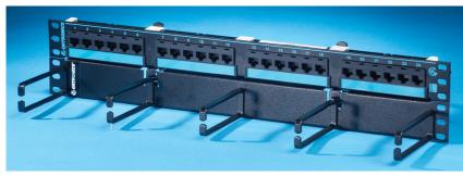
Clarity 6 24-port high density patch panel with hinged cable management panel is component compliant to TIA/EIA Category 6 performance requirements. It occupies two rack units, and measures 19" x 3.5". Jacks are grouped in six-port modules. It is part of the Clarity 6 link and channel solution that provides significant installed performance headroom.
