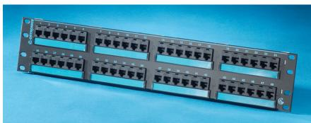
Clarity 6 48-port high density Category 6 patch panel is component compliant to EIA/TIA Category 6 performance requirements. It occupies two rack units, and measures 19" x 3.5". Jacks are grouped in six-port modules. Part of the Clarity 6 link and channel solution that provides significant installed performance headroom.
