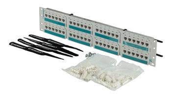
Clarity 6 48-port high density Category 6 patch panel is component compliant to EIA/TIA Category 6 performance requirements. White panel occupies two rack units, and measures 19" x 3.5". Jacks are grouped in sixport modules. Part of the Clarity 6 link and channel solution that provides significant installed performance headroom.
