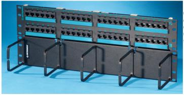
Clarity 6 48-port high density patch panel with hinged cable management panel is component compliant to TIA/EIA Category 6 performance requirements. It occupies four rack units, and measures 19" x 7.0". Jacks are grouped in six-port modules. It is part of the Clarity 6 link and channel solution that provides significant installed performance headroom.
