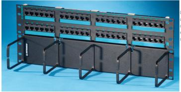
Clarity 6 48-port high density patch panel with hinged cable management panel is component compliant to TIA/EIA Category 6 performance requirements. It occupies four rack units, and measures 19" x 7.0". Jacks are grouped in six-port modules. It is part of the Clarity 6 link and channel solution that provides significant installed performance headroom.
