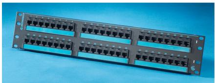
Clarity 6 48-Port High Density Category 6 patch panel is component compliant to EIA/TIA Category 6 performance requirements. It occupies two rack units and measures 19" x 3.5". Jacks are grouped in eight-port modules. Part of the Clarity 6 link and channel solution that provides significant installed performance headroom.
