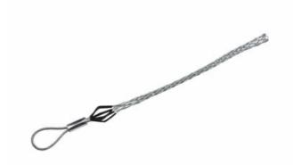
Junior Duty, Flexible Eye. Cable Diameter - 0.250-0.360-inch, Mesh length - 5-inch, Break Strength - 1,700 lbs.
