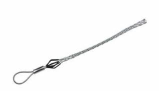
Junior Duty, Flexible Eye. Cable Diameter - 0.250-0.360-inch, Mesh length - 5-inch, Break Strength - 1,700 lbs.
