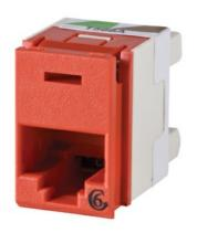
Clarity 6 patch panel jacks, rear load into patch panels and exceed Category 6 component specifications. Rear load positive latch design, secures mounting of the jack into the patch panel. Universal T568A/B wiring label and tapered wiring towers simplify termination.
