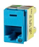
Clarity 6A patch panel jacks, rear load into patch panels and exceed Category 6a component specifications. Rear load positive latch design, secures mounting of the jack into the patch panel. Universal T568A/B wiring label and tapered wiring towers simplify termination.
