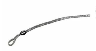
Medium Duty, Short Length, Flexible Eye, T-Type. Cable Diameter - 0.750-0.990-inch, Mesh Length - 24-inch, Eye Diameter - 1/4-inch, Break Strength - 6,800 lbs.
