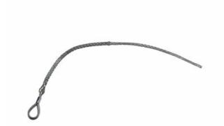
Medium duty, Long length, Flexible eye. Cable Diameter - 1.000-1.490-inch, Mesh length - 48-inch, Break Strength - 11,600 lbs.
