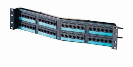
Clarity® SNAP patch panels offer improved rear cable management with the addition of an adjustable depth rear management bar. The rear portion of these bars is also removable to provide more working room for the initial termination of panels. After cables are SNAP terminated, the rear bars are attached and adjusted to the depth that best matches the cable and rack selections.
