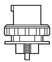
Triple-Pole, 4-Wire, Pin and Sleeve Watertight Inlet. 125A, 200/250V.
