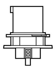
4-Pole, 5-Wire, Pin and Sleeve Inlet. 20A, 3Y, 120/208V.
