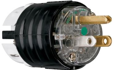
Straight Blade Hospital Grade Plug, double pole andthree wire, unit arrives completely ready-to-wire, cutting installation time significantly. Its nylon housing provides impact and chemical resistance. Its rugged two-piece cord grip provides more uniform cord retention and the internal dust shield keeps terminals free of contaminants. 15amp 125volt.
