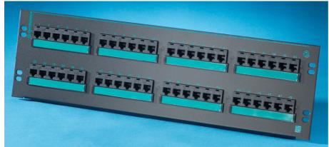
Clarity 5E 48-Port Patch Panel is component compliant to EIA/TIA Category 5e performance requirements. Standard density design provides additional space for cabling and occupies three rack units, measuring 19" x 5.25". Jacks are grouped in six-port modules. Part of the Clarity 5E link and channel solution that provides significant installed performance headroom.
