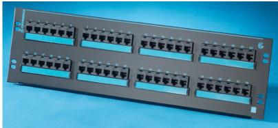
Clarity 6 48-Port Category 6 patch panel is component compliant to EIA/TIA Category 6 performance requirements. Standard density design provides additional space for cabling and occupies three rack units, 19'' x 5.25''. Jacks are grouped in six-port modules. Part of the Clarity 6 link and channel solution that provides significant installed performance headroom.
