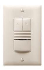
The PW-311 passive infrared (PIR) dimming wall switch sensor can turn lights OFF and ON based on occupancy and allow the user to increase or decrease the lighting level. It works with 0-10 VDC dimming drivers and ballasts to control lighting loads including LEDs.
