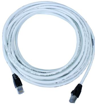
PWC5E PowerWise Cat5E UTP solid 22 awg conductor plenum, double ended 10ft, white
