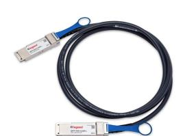
5m Cisco QSFP-100G-CU5M Compatible 100GBase-DAC QSFP28 to QSFP28 (Passive Twinax Copper, PVC) Direct Attach Cable
