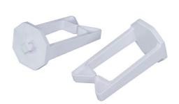
Cable retention ring kit consists of 4 rings to improve cable management from the overhead pathway racks. The rings have a quarter turn feature which makes them easy to install, even after the rack has been deployed. The rings can mount to the front surface as well as the side surfaces of the rack.
