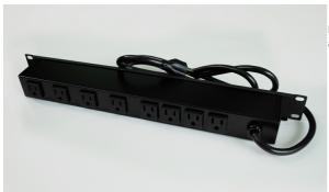
Eight rear outlets, lighted switch, 15A. Receptacles rotated 90 degrees and 4 outlets spaced to accommodate transformers. 6' (1.8m) cord. Perma Power computer grade surge protection.
