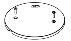
Available in black (BK), and gray (GY). NOTE: To abandon the RC3 Series Poke-Thru Device, the duplex receptacle must not be removed in order to maintain UL Classification. Also the stem must remain in the hole.
