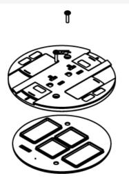
Nonmetallic slide holder assembly. Available in black (BK), gray (GY), ivory (VY), nonmetallic brass (BS), and nonmetallic aluminum (AA). Assembled with scrub water gasket. For use on tile or carpet floors.
