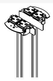
Prewired snap-in 20A receptacle can be wired as standard duplex or isolated ground. Available only in black. See installation instructions with replacement receptacle for complete installation details.
