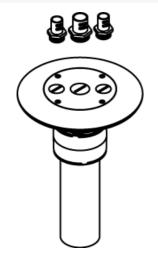
2" trade size conduit stem, complete with one 3/4" trade size conduit and two 1/2" trade size adapters and closure plugs. Finish flange/cover assembly available in painted gray (GY), black (BK), brushed plated brass (BS), and brushed aluminum (AL). NOTE: Assembled with scrub water gasket. For use on tile or carpet floors. RC9AM2TC Series Poke-Thru Devices require a 3" (76mm) diameter hole. Not designed to work with bare concrete or terrazzo. Floor covering thickness 1/8" minimum.
