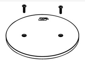
Abandonment available in black (BK) or gray (GY). NOTE: To abandon the RC7 Series Poke-Thru Device, the internal gasket, duplex receptacle, and communication modules must not be removed in order to maintain UL Classification. Also the stem must remain in the hole.
