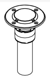
Use with RC9CMD and RC9AM2TC Series Covers to complete installation. NOTE: RC9AMD and RC9AM2TC Series Poke-Thru Devices require a 3" (76mm) diameter hole. Not designed to work with bare concrete or terrazzo. Floor covering thickness 1/8" minimum.
