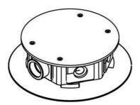
Complete with gray or black carpet flange, gray hexagonal housing, five black rubber grommets, and one 3/4" trade size threaded dropin hub. The service head includes scrub water gasket. Colors available in painted gray (GY), and black (BK). Use with the RC9FFS Insert to form a complete poke-thru assembly. NOTE: RC9AFFTC Series Poke-Thru Devices require a 3" (76mm) diameter hole. Not designed to work with bare concrete or terrazzo. Floor covering thickness 1/8" minimum.
