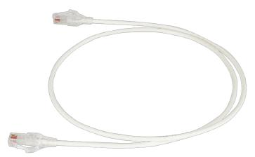
RDC 6 Modular Patch Cord, white, 5', reduced diameter, 28 AWG, cat6 channel four-pair UTP stranded PVC/CM.
