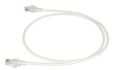
RDC 6 Modular Patch Cord, white, 10', reduced diameter, 28 AWG, cat6 channel four-pair UTP stranded PVC/CM.
