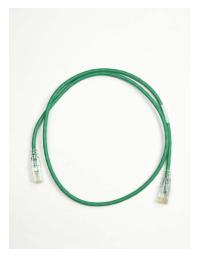
The RDC610 series of modular patch cords offer the reduced diameter of four pairs of 28AWG conductors, providing CAT6A channel performance for high density applications, when looking to reduce congestion or improve airflow through cabling pathways. Common applications include high-density cabling areas such as data centers, end-of-row (EoR) and top-of-rack (ToR) installations or areas such as telecom rooms and equipment rooms.
