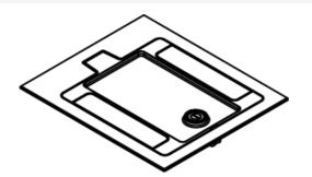
Cast aluminum cover assembly available in brushed aluminum (AL), painted black (BK), and gray (GY). Provided with carpet cut-out area. Maximum load capacity 1,500 lbs. UL Listed to U.S. and Canadian safety standards to meet UL requirements under UL514A for scrub water exclusion. NOTE: Not for use on bare concrete floor applications.
