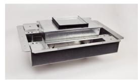
Fire Classified 2-Compartment Box. For use in either concrete or wood floors. Fully adjustable with tunnel compartment. Supplied with one (1) duplex receptacle mounting plate, and one (1) communication mounting plate (RFB22AB). Other device plates sold separately. This floor box preserves the 3-hour fire rating of floors in which it has been installed.
