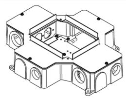
14 1/2" L x 11 7/8" W x 3 7/16" D (368mm x 302mm x 87mm). Fully adjustable with tunnel compartment and two receptacle brackets. Feed through from adjacent or opposite compartments only, (not cross compartments). Communication brackets not included. Note: Only for use in concrete floors. All boxes and activations are sold separately.
