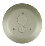
Kit comes complete with adapter ring to secure into the boxes, [1] 3/4" trade size screw plug and conduit fitting for power, 1-1/4" trade size screw plug and conduit fitting for low voltage (communications or Audio/Video) services.
