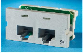
Clarity 5E Series II module two jack ports (1 unit), ETL verified to TIA Category 5e component specification. Front-loading and front removable. New universal T568A/B wiring label and tapered wiring towers simplify termination. Center tuned to Clarity 5E patch cords for optimum performance.
