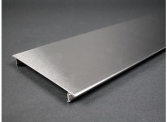
.040" (1.0mm) stainless steel. Snap-on cover for mounting 4 1/2" (114mm) device plates on 36" (915mm) centers.
