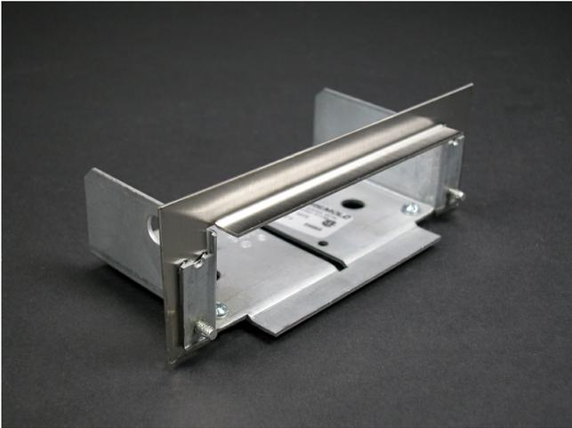
To connect S4000 Series Raceway with surface type panel boxes. Accommodates maximum wire capacity of S4000 Series Raceway. Separate C-shaped flange fits around raceway, covering any irregularities from cutting into box. Cut 4 3/4" x 1 3/4" (121mm x 44mm) hole in panel box.
