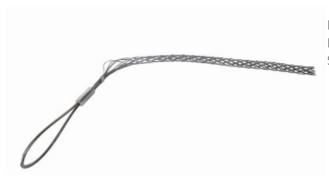
Double Weave, Standard Length, Closed Mesh, Offset Eye. Cable Diameter - 1.000-1.240-inch, Mesh Length - 16-inch, Break Strength - 4,200 lbs.
