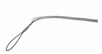
Double Weave, Standard Length, Closed Mesh, Offset Eye. Cable Diameter - 1.500-1.740-inch, Mesh Length - 18-inch, Break Strength - 7,400 lbs.
