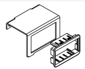
Single-gang adapter. Includes one (1) Wiremold Open System adapter.
