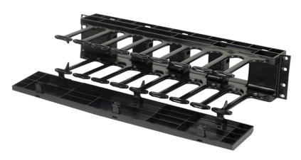
Horizontal cable managers are available in 1RU, 2RU, 3RU, and 4RU sizes. Fingers begin 3/4 in from the face of rack to provide bend limitation for cables, protecting cables, equipment and network performance. Included hinged cover mounts with six heavy duty clips allow them to be opened one handed without becoming "unhinged". Manufactured from UL94V-0 rated
